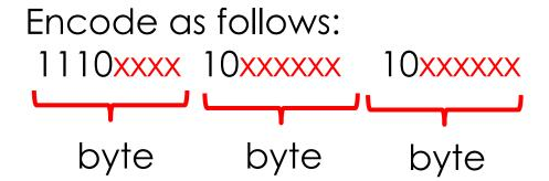
Decoding (mapping a sequence of bytes to characters):
