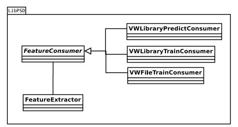
Figure 6: UML diagram of the PSD library.
